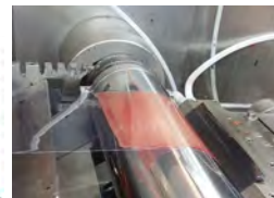
Lamination of solvent-cast polymer/QD matrix onto carrier film
